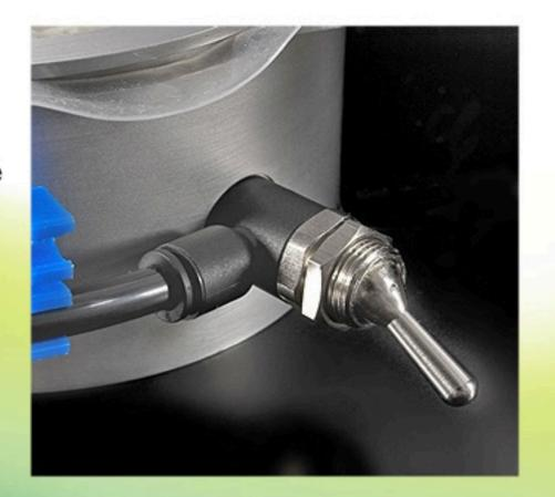
7. When the gasket is in place, move the switch to the closed position to maintain the vacuum during the curing stage.
