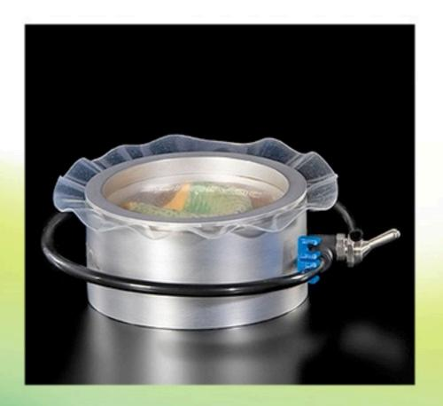
2. Remove the metal o-ring, and the reusable silicone gasket.
