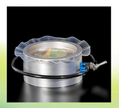
5. Insert the free end of the black tubing attached to the main body of the EZ VAC into the hand pump.
