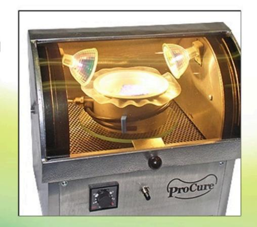
3. When curing is completed turn off the light curing unit and remove the EZ VAC.
