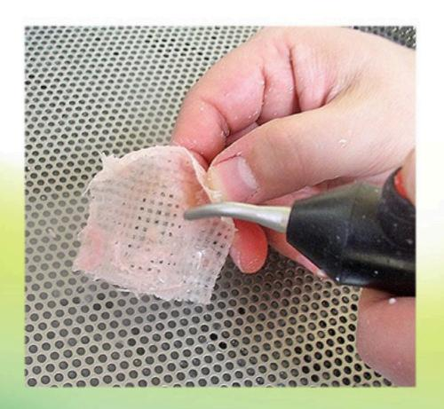
Using scissors trim the mesh matrix to the final desired shape and size.
